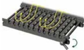
**OPEN POSITION** for smokeless fuels - allowing the air to flow up through the fuel. In this position the open bars facilitate easy ash removal whether burning wood or solid fuel products.
